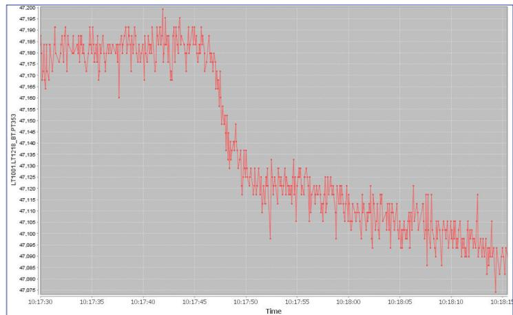
**Fig.10. The resolution of new pressure measurement (vertical axis indicates pressure in the pipeline), bar.**
