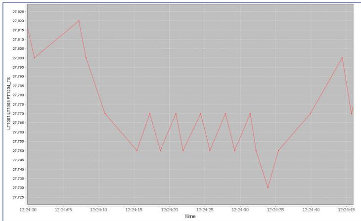
**Fig.9. Resolution of pressure measurement (vertical axis indicates pressure in the pipeline), bar.**
