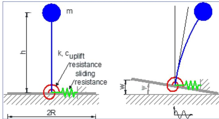
Fig.8. Spring-mass model of the tank.
