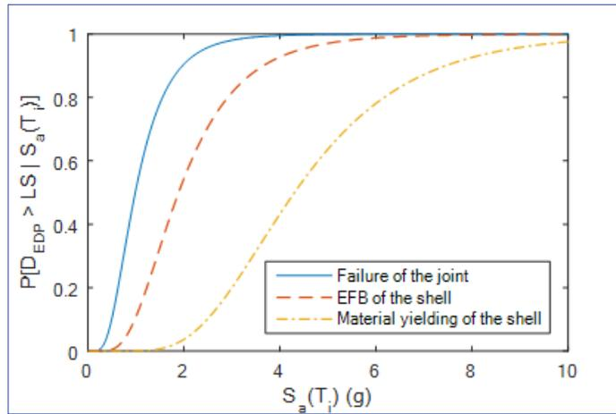
**Fig.11. Fragility curves of the tank.**
