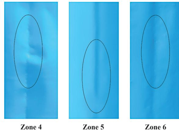
Figure 2. Zones selected for the analysis of changes in surface equivalent stress of VSTP-20000 tank.
