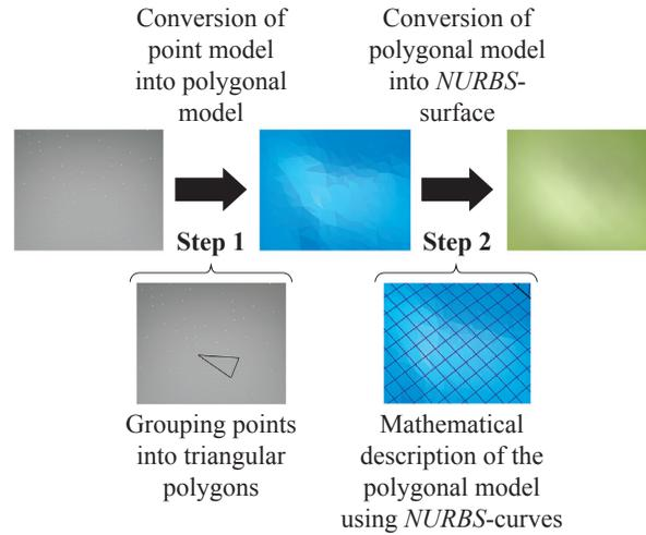
Figure 1. The procedure of converting a point model into a 3D mathematical model.
