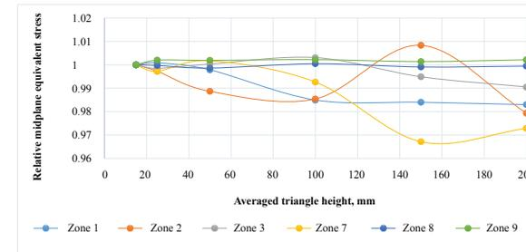
Figure 5. Relative change of the midplane stress in the tank wall (stress at  $h = 15$  mm is taken equal to 1).
