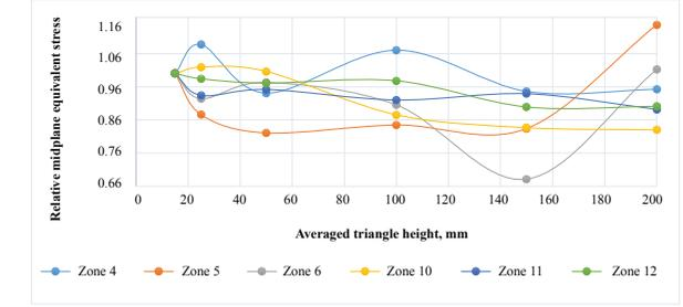
Figure 6. Relative change of the surface stress in the tank wall (stress at  $h = 15$  mm is taken equal to 1).
