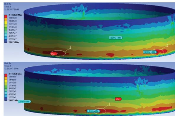
Figure 3. Midplane equivalent stress in VSTP-20000 tank wall at  $h = 15$ .
