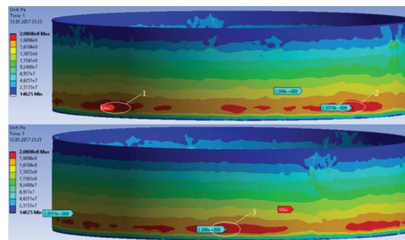
Figure 4. Midplane equivalent stress in VSTP-20000 tank wall at  $h = 200$  mm.
