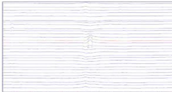
Figure 12. Liffoff Data (LRC) showing sensor liffoff > 1.5mm for Dents 3-5.
