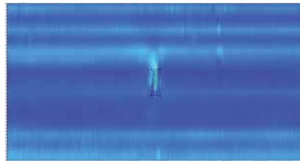
Figure 15. MFL metal loss data with internal discrimination channels in background color scan for Dent 13.
