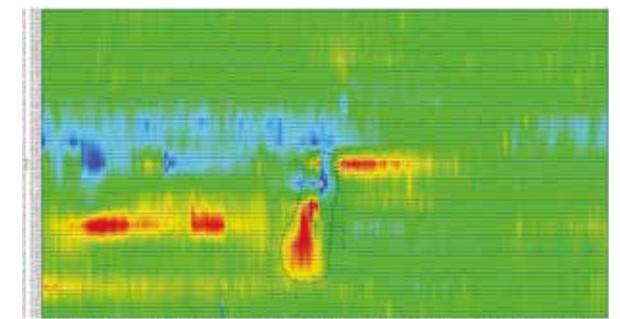
Figure 8. Liftoff data (LRC) showing sensor liftoff > 1.5mm for Dent 11.
