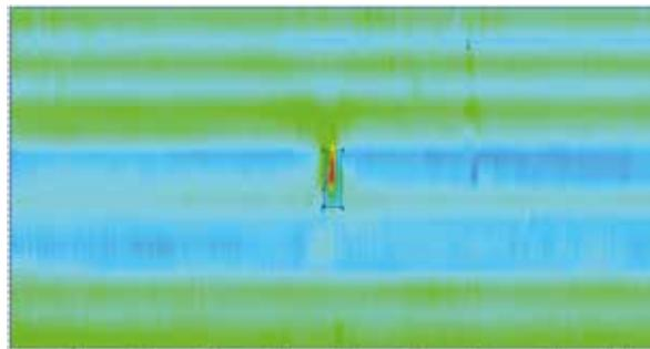
Figure 14. MFL metal loss data showing interaction between dent and metal loss call boxes for Dent 13.
