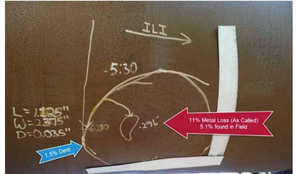
Figure 1. Example dent with minor metal loss.
