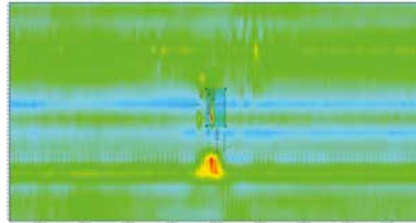
Figure 11. MFL data confirming metal loss interaction for Dents 3 to 5.
