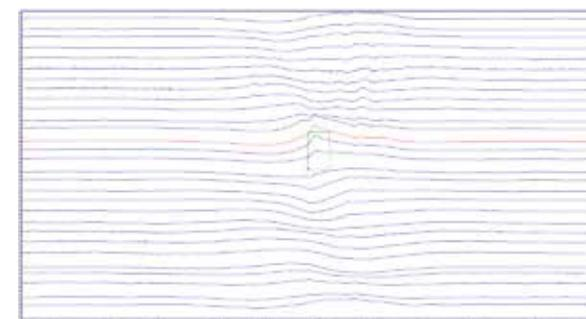
Figure 9. Liftoff data (LRC) with adjusted scale showing liftoff < 4.5 mm for Dent 11.
