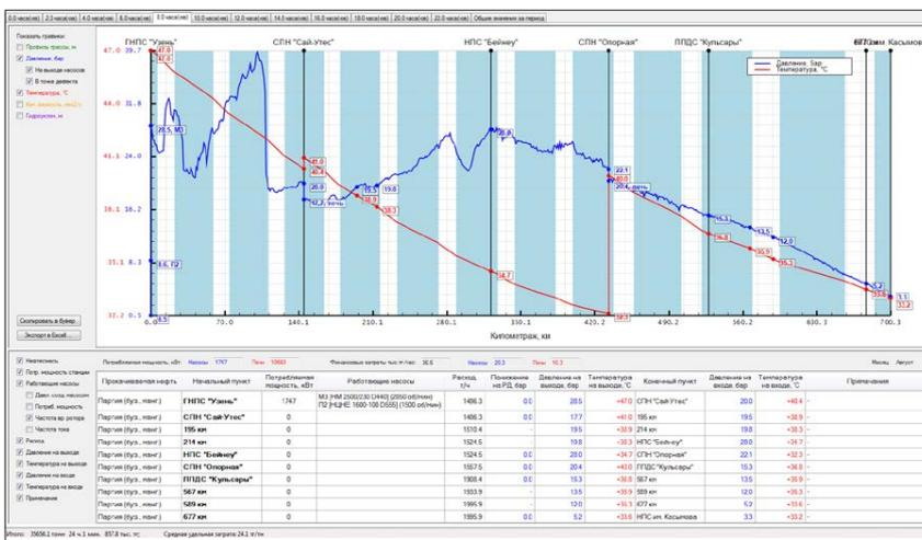
Fig.9. Calculation data for pressure and temperature in the period from 08:00 to 10:00 when batch pumping Buzachi and Mangyshlak oil blends at the Uzen-Atyrau section with soil temperature for August.
